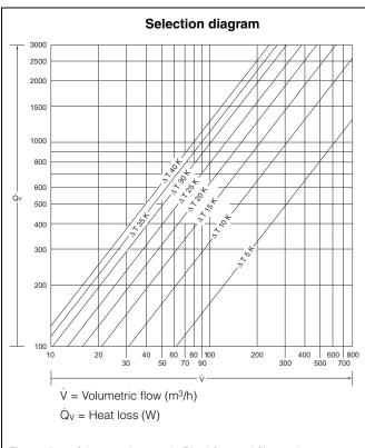
The styling of the vent louvres in Rittal fan-and-filter units guarantees exemplary stability of the air volumes in relation to pressure loss. The correct fan-and-filter unit has been chosen if the specified heat loss is dissipated whilst complying with the desired maximum enclosure internal temperature.
