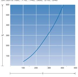
$\dot{V}$  = Volumetric flow (I/h)  $\Delta P$  = Water resistance (mbar)
