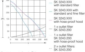
$\dot{V}$  = Volumetric flow (m<sup>3</sup>/h)  $\Delta P_{st}$  = Stat. pressure difference (Pa)
