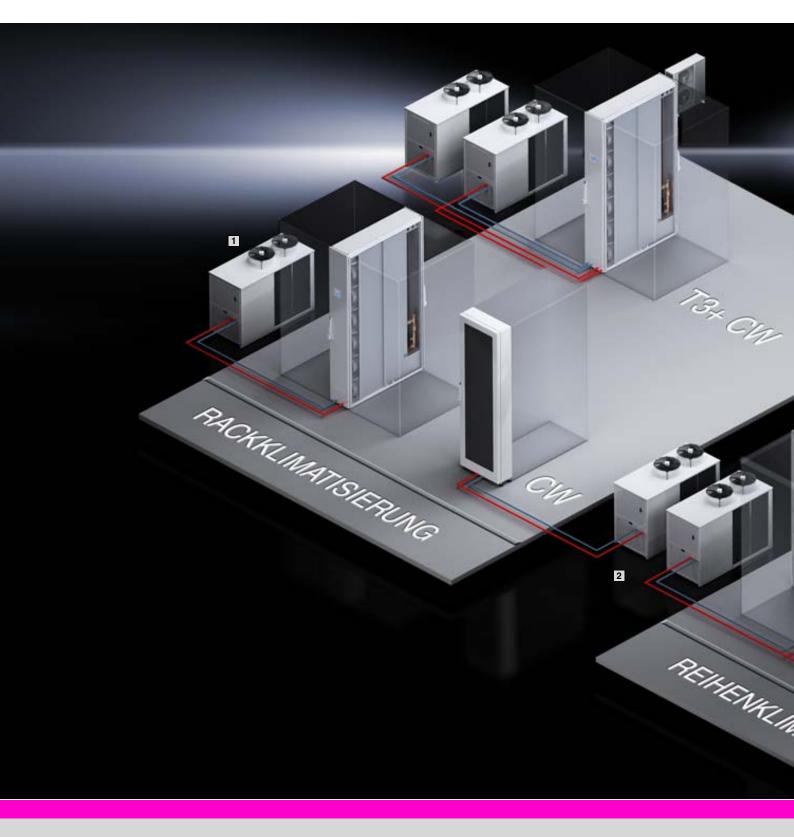
Climate control of your data centre is becoming ever more important in terms of availability and energy costs. The Rittal Liquid Cooling concepts ensure precise, problemfree heat loss dissipation of up to 60 kW per rack.
