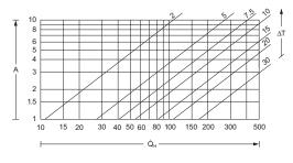
$\dot{Q}_{H}$  = Thermal output (W) A = Enclosure surface area to IEC 890 (m<sup>2</sup>)  $\Delta T$  = Temperature difference (K)
