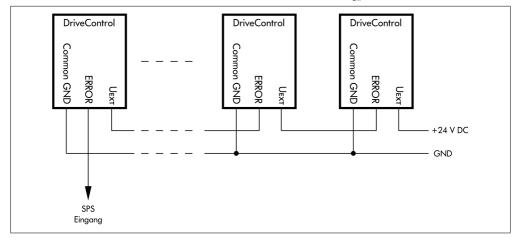
When the operating voltage is switched off, the ERROR output will switch to the "error" state. This guarantees a correct error message even when the error signal has been linked from multiple DriveControl units and the operating voltage of a DriveControl unit is switched off, or a cable error has occurred (detached contact, cable break).
