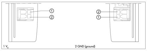
The power supply connection features a double-sided design, meaning the most favourable side (in terms of installation) can be used to connect the power supply. Both connections are directly internally linked with one another. The power supply can be fed through a DriveControl, allowing a maximum of two DriveControl units to be connected in succession.
