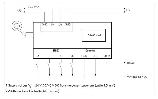
For issue-free connection to a PLC, we recommend a separately conducted control voltage  $V_{_{EXT}}$  of 24 V DC.
