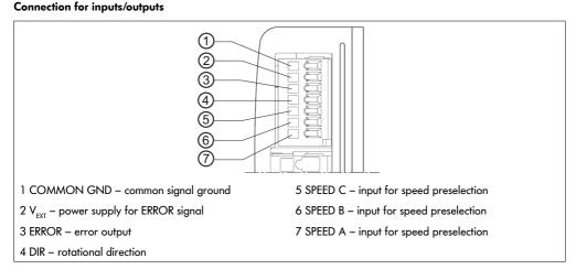
V<sub>FXT</sub> typically corresponds to +24 V DC (max. +55 V DC).
