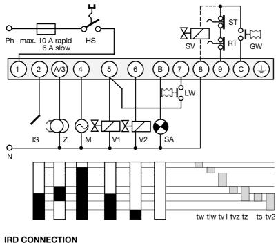
ST Limit thermostat Control thermostat RT IS Ionization probe Ignition Ζ Μ Burner motor V1 Solenoid valve 1st stage V2 Solenoid valve 2nd stage LW Air pressure monitor External fault indication SA SV Safety valve Waiting time at start-up tw Max. reaction time tlw for air proving switch tv1 Pre-purge time Pre-ignition time tvz tz Total ignition time Safety time ts tv2 Time delay term.6 / term.C
