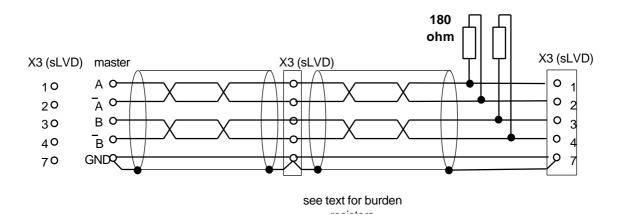
In the example given above, the connection of two SLVDs to the Digital-Lock with a master is shown, but the diagram could be extended to several converters respecting the series connection. The line charge resistors must be connected to the last converter. The master can be an encoder powered externally or an encoder simulator of another converter.
