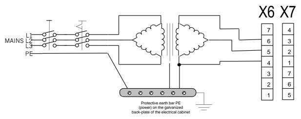
Use of a transformer connected in a star configuration with a primary and secondary electrostatic shield
