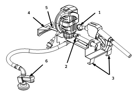
Insert the drip collection pipe (1) included in the scope of the delivery into the mounting hole on the bracket.
