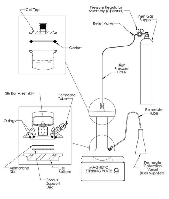
Figure 5: HP4750X Stirred Cell System Schematic
