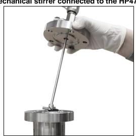
Figure 3: Mechanical stirrer connected to the HP4750X cell top
