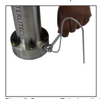
Photo 7: Permeate Tube Installation
