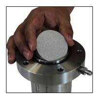
Photo 4: Membrane Support Disk Insertion
