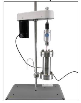
Figure 4: HP4750X cells assembly with mechanical stirrer
