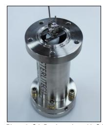
Photo 8: Stir Bar Insertion with Stir Bar Retriever
