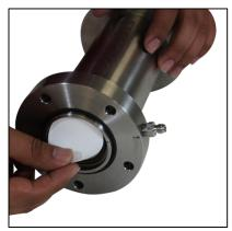
Photo 3: Membrane Filter Insertion
