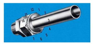
3. Hold the fitting body steady with a backup wrench and tighten the nut 11/4 turns. Watch the scribe mark, make one complete revolution and continue to the 9 o'clock position. When the nut is tightened to the 9 o'clock, you can easily see the fitting has been tightened properly.
