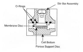
9. Insert the gasket on the top of the Cell Body, making sure it fits properly in the grooves (Photo 9).
