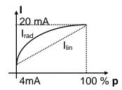
The S1 sliding switch (see fig. 1) allows the operator to toggle between a root-extracted and linear curve.
