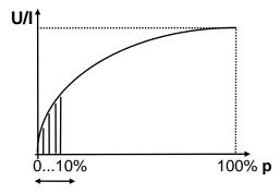
The creep-suppression function suppresses the pressure transducer output, i.e., keeps it at "0", despite any existing pressure. The P5 trimmer can be used to set creep suppression to a value between 0 and 10% of the measurement range. Use of the creep-suppression function is advisable for many applications, as the instrument will otherwise fail to generate reproducible results of a measurement when the flow rate / volume flow is very low.
