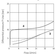
**3** = A  $\rightarrow$  T (dotted line for pressure range /350) **4** = Pressure drops vs. flow P n A
