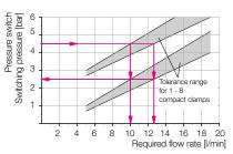
Required flow rate depending on the switching pressure of the pneumatic pressure switch for a pressure drop  $\Delta p$  2 bar
