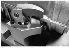
Clamping of a cast part
