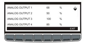
This outputs can be used to drive an external inverter or to repeat a main probe, by means of a signal 4-20mA or 0-10V.
