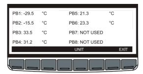
To change the measurement unit for the probe PB1, PB2, PB3, PB4, push UNIT button.
