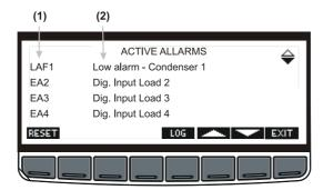
The alarm menu displays the active alarm with the following layout:
