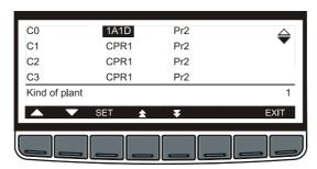
Push the key and use the **UP** and **DOWN** keys to modify the value.
