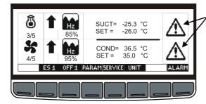
If the alarm icon is flashing on the main display, an alarm is occurring.
