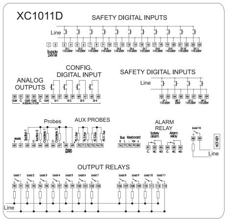
**NOTE**: according to the models the **digital inputs**: (3-24) and (52-59) can operates at 230V/120V or 24V. Verify on the controller which is the right voltage that can be applied.
