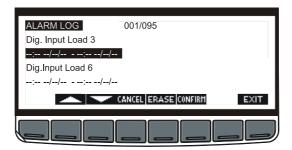
Push the **CONFIRM button** to confirm the operation and delete the archive. Push the **CANCEL button** to cancel the operation and come back to the ALARM LOG menu.
