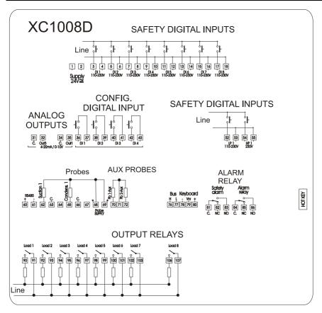
**NOTE**: according to the models the **digital inputs**: (3-18) and (52-55) can operates at 230V/120V or 24V. Verify on the controller which is the right voltage that can be applied.
