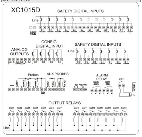
**NOTE**: according to the models the **digital inputs**: (3-26) and (46-59) can operates at 230V/120V or 24V. Verify on the controller which is the right voltage that can be applied.
