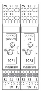
Figure 7. Coolant (TCR1) and oil (TCR3) control TCR showing terminals T1 (blue wire), T2 (brown wire) and T3 (black wire).
