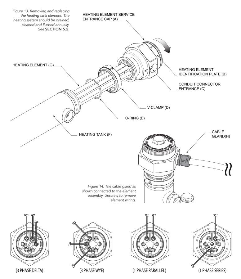
Figure 15. Heating tank element phase configurations. Replacement elements may be a different phase configuration.
