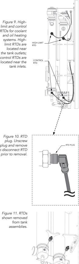
Figure 10. RTD plug. Unscrew plug and remove to disconnect RTD
