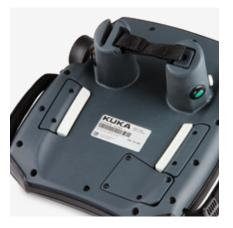
Elements for ergonomic left- and right-handed operation and a service flap for simple cable exchange round off the user-friendly design of the KUKA smartPAD.
