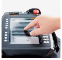
Efficient operation with brilliant, capacitive touch display. Inputs are made quickly and easily via the 8 4" screen
