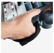
Comfortable, relaxed handling. The new KUKA smartPAD features impressively pleasant handling. Straps and handgrips that can be used with both hands greatly simplify operator control. An optional shoulder strap enables work without tiring the operator – particularly during time-intensive projects.
