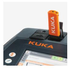
State-of-the-art hardware. Thanks to the latest hardware, the KUKA smartPAD impresses with strong performance. Two easily accessible USB ports enable direct saving and loading of application programs and connection of other supported USB devices.
