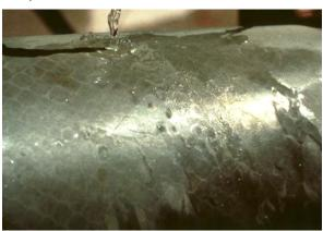
6. If any portion of the PTFE coated screen is wetted by the water (the water will seep into the pores of the screen; this is very obvious to the eye), the cartridge has failed the Water Test. The wetted area must be cleaned again (see Step 7), and the recleaned cartridge should pass the Water Test before it is reinstalled.
