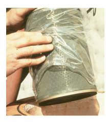
2. After removing the cartridge from the vessel, submerge it in clean fuel and gently scrub the entire screen surface with a soft bristle brush or a lint free cloth.
