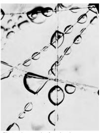
Photomicrograph of coalescing process inside fiberglass media.
