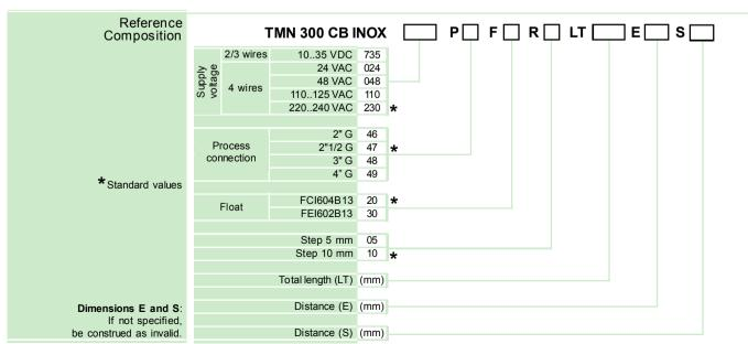
To compose a reference, select an option from each of the columns. Example: TMN 300 CB INOX 230 P47 F20 R10 LT1500 E15 S75
