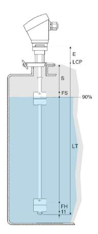
You can determine a bound (S) to establish an area where there is no reading at all. In case you want to remove the head of the connection process (for reasons of high temperature, for example) may specify a dimension (E) exceeding the standard.
