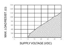
**Supply in AC:** The electronic circuit provides a voltage of 24 VDC to power the loop. The load resistor should not exceed 800 ohms.
