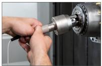
Easy to operate The force sensing bar is inserted into the tool machine spindle and tightened.
