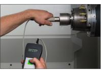
Accurate readout The pull force is transmitted by an electrical measuring signal to the readout unit and can be read off there.
