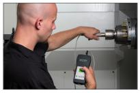
Fast reading A precision force sensing bar with expansion measuring strips performs the measurement.
