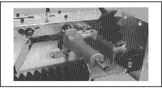
**Trolley Assemblies –** lubricant injector (coupler), trolley wheel locator and control to synchronize lubricator operation with conveyor movement.
