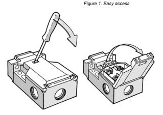
Access the wiring chamber via a hinged door. Simply insert a flat-blade screwdriver, as shown, and pry gently down to open.
