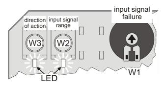
Fig. 1. Pushbuttons and potentiometer (default positions)
