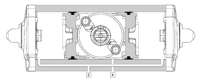
The port 2 is in connection with the cylinder side chambers, supplying the pressurised air in port 2 the standard Double Acting actuator drive shaft rotates counter clockwise to open , while the port 4 is in connection with the intermediate chamber and when pressurised the drive shaft rotates clockwise to close.
