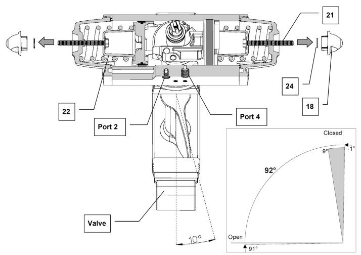
\*\*\*WARNING: The Spring Return close adjustment is not a mechanical stop that act against the pistons travel or the shaft rotation, but the screws limits the spring travel and the pistons without any force standstills. In this condition the shaft is not stopped and theoretically could be moved to the total closing position, adjustments of closing and opening can not be performed both. OMAL standard stroke adjustment is max 10°, special longer screws are available on request.
