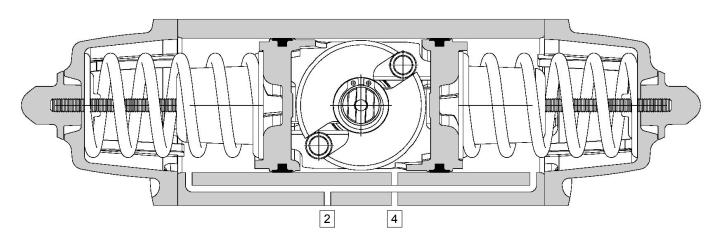
The port 4 is in connection with the intermediate chamber and when pressurised the drive shaft rotate counter clockwise to open.
