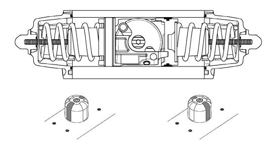
Simple Acting Spring Return fail to open operation cycle.
