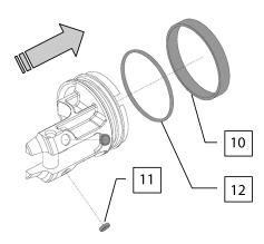
a.4) When the components are disassembled, they should be properly cleaned and wear checked prior to being greased and reassembled. In case the sealing parts are too much worn out use new parts from the spare parts kit.
