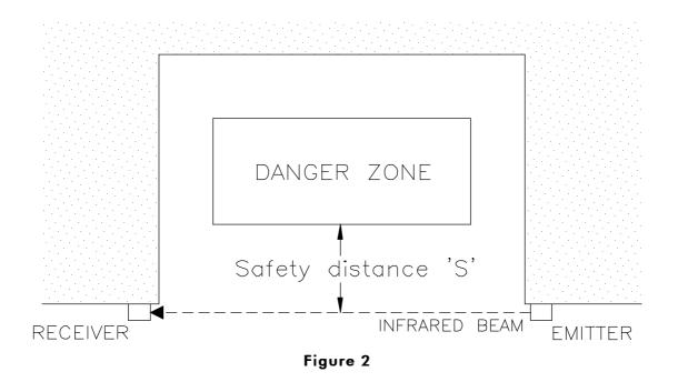
With reference to the proposed European standard prEN999, the minimum safety distance, S, must be calculated through the following formula:
