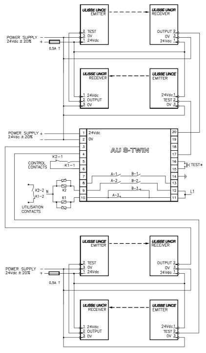
Connection of four pairs of photocells with AU S-TWIN and with auxiliary external relays K1 and K2 control.
