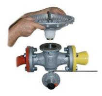
11) Separate the balancing group (200) from the head (300) by modifying the flowing-direction of the gas in order to get the shaft (203) getting out of the loading joint (312);
