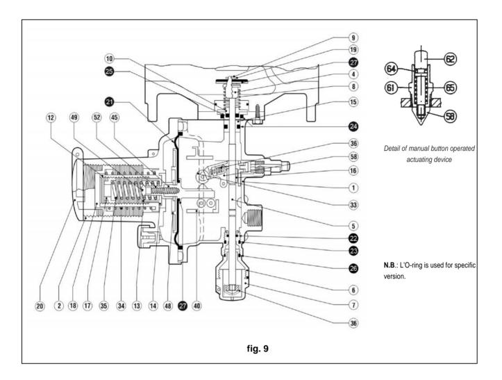
The slam-shut valve LA.. consists essentially of an obturator (fig. 9) fitted on a stem, a releasing lever system, a control head and a manual resetting system. The pressure to control Pd, in chamber C of the control head, acts on the diaphragm 46 which is integral with the cam shaft 45.
