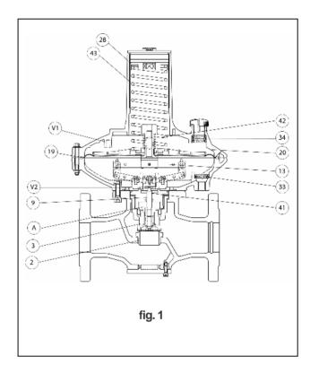
In fact, this solution allows the diaphragm protection disc  $20\,\mathrm{to}$  rest on the upper stroke end V1 exceeding the load of the spring  $42\,\mathrm{and}$  thus releasing the obturator from the load resulting from the sudden pressure increase.
