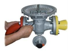
10) Separate the head (300) and the balancing group (200) from the regulator's body (1);
