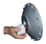
Unscrew the screw (212) from the obturator (211) and separate all the components of the balancing group (200);
