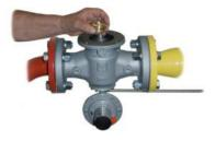
Unscrew then the screws (48) to dismantle the lower blind flange (10). To re-install the regulator you can carry out the operations described for the dismantling, in the opposite way.
