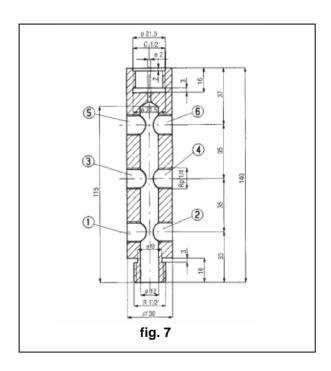
The installation of a multiple plug on a plant has its aim in in taking from a single point all the pressure impulse signals that go to the different reduction- safety devices and to their accessories.
