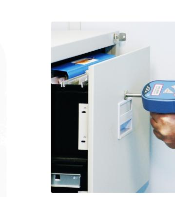
Captures peak readings in tension or compression
