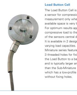
a sensor for compression measurement only where the available space is very limited. For optimum results apply compressive load to the top of the sensors central dome. It is available in 2 designs and varying load capacities. The Miniature series features 3 threaded holes for fixing the Load Button to a base and is typically larger and taller than the Sub-Miniature series which has a low-profile design without fixing holes.
